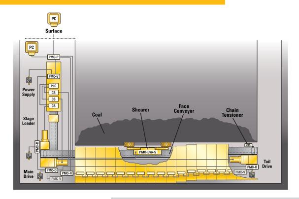
The PMC system offers a tailored control unit for each of the various longwall functions:
