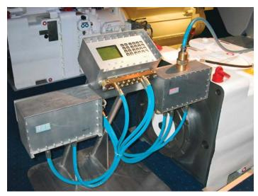
Configuration of PMC-D and PMC-V connected to a CST drive
