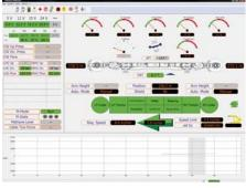
**VDrive** – Visualizes the conveyor gearbox controllers. A range of sensor values can be displayed graphically and all parameters can be changed.
